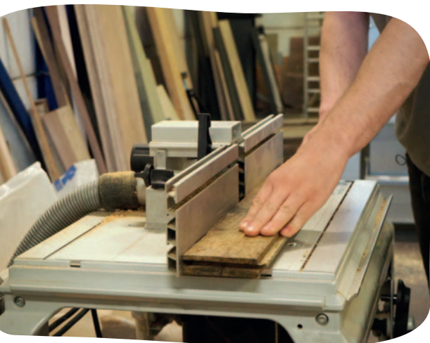
Cleaning of the groove in parquet strips, after cutting, to adapt their size to their new purpose.
